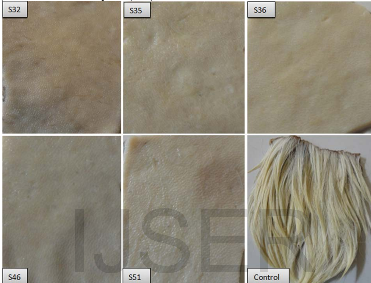
Figure 3: Completely dehaired goat skins by crude proteases of 5 isolates (S32, S35, S36, S46, and S51) at 40°C for 6 h; (control) skin treated with only buffer of pH 10.
